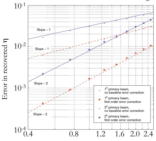
Antenna position errors in units of  $\lambda$
