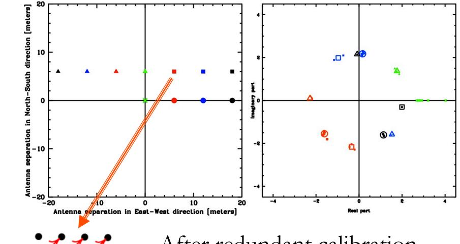
After redundant calibration, redundant baselines give identical results
